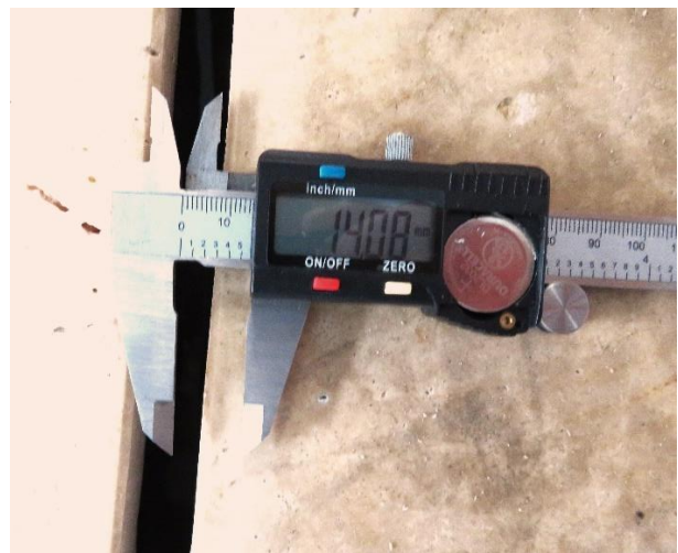
Plate 2: 14mm wide single overflow slot.
